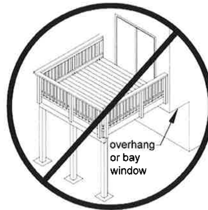
Figure 18. No Attachment to House Overhang with Ledger.
